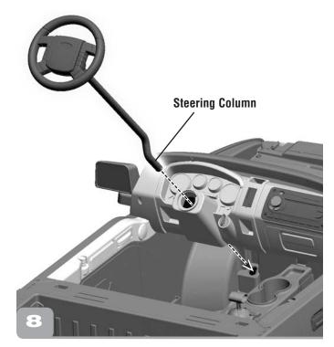
Insert the end of the steering column down through the opening in the dash and down through the hole in the vehicle floor.
